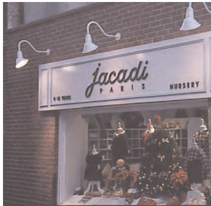
Another example of goose neck exterior wall-mounted fixtures that focus on illuminating the store's sign. Note also that the display windows are well lit.
