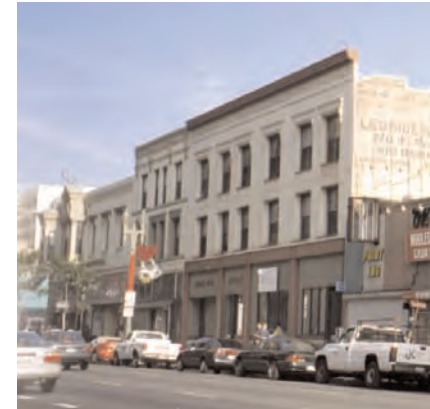
Main Street rhythms are created by similarly placed and spaced window openings and continuous horizontal lines.
